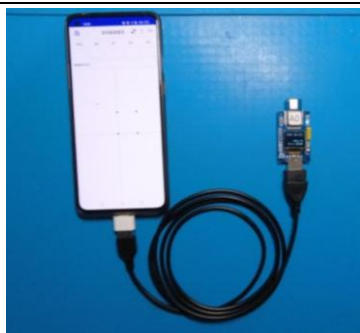
Figure 6-1 RTLS1 Module Connects to Android Phone
