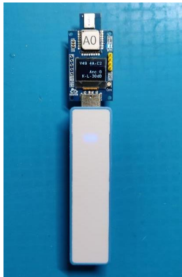
Figure 5-2 ULM1/3 Module Connects to a power Bank
